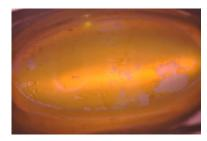
21. Coloured layer with chipped off areas was readily visible at the base of these sillimanite cabochons.
