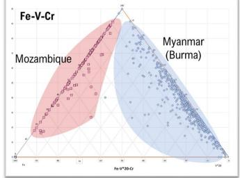
5. Ternary plot, such as this comparing ratio of Fe-V-Cr is useful in separating rubies from Myanmar (low iron) and Mozambique (high iron).
