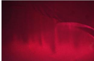
**29.** The 65.14ct rough displayed curved clouds of minute gas bubbles, confirming its synthetic origin, grown by Verneuil process.
