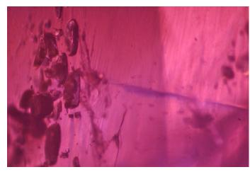
**17.** The 12.08ct pink sapphire displayed blue and yellow colour flashes along fissures suggesting presence of high RI glass. Also note the cluster of crystals with slightly corroded surface.
