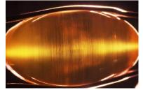
20. Such fine parallel needles or fibres causing chatoyancy is commonly seen in sillimanite.
