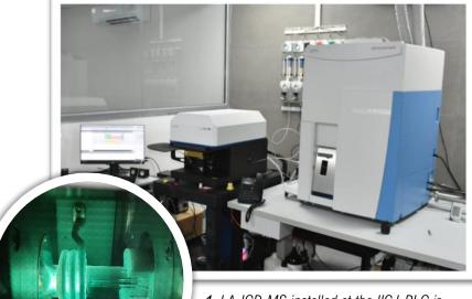
**1.** LA-ICP-MS installed at the IIGJ-RLC is extensively used for detailed chemical fingerprinting, before issuing reports on origin.
