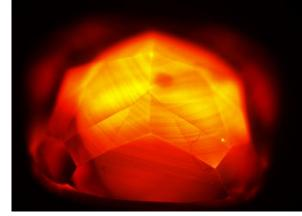
**24.** Typical example of striated growth pattern in CVD grown diamonds, along with orange fluorescence.
