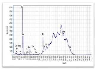
**18.** Presence of bromine (Br) in this filled sapphire was confirmed with EDXRF spectroscopy.
