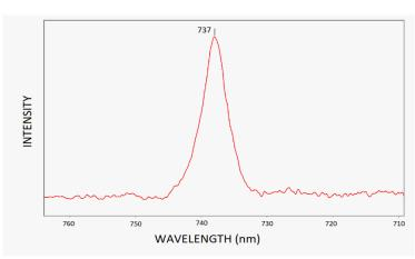
**25.** Photoluminescence spectrum displaying feature at ~737nm, characteristic for CVD grown diamonds.
