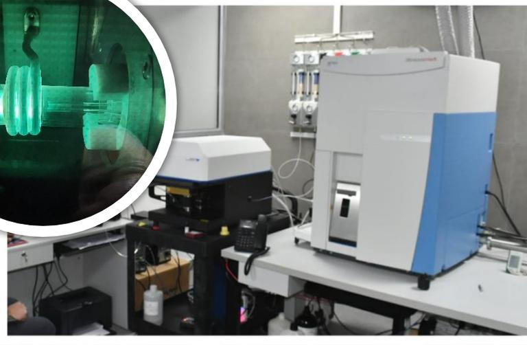
4. LA-ICPMS installed at the IIGJ-RLC is extensively used for detailed chemical fingerprinting, before issuing reports on origin of emeralds.
