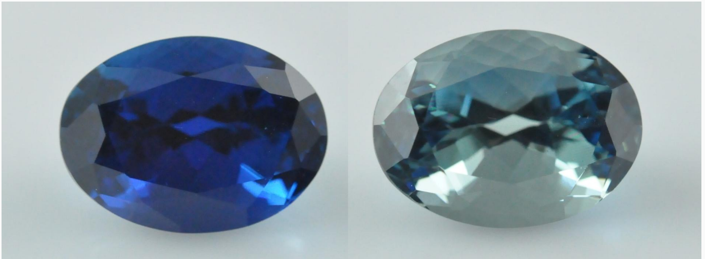
Figure 2: The dichroic aquamarine displayed unusually intense dichroism, with a deep saturated blue along the e-ray (left) and a pale bluish green along the o-ray (right). The images were taken by fixing the polarizing filter on the camera lens and rotating the polarizer 90 degrees to separate out the two directions.
