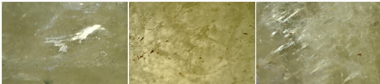
Figure 2: Examination of the carving with a hand loupe revealed reflective liquid films (left), elongated phase/short tubes oriented in one direction and aligned in planes intersecting each other at approximately 65/115° (center), and parallel reflective films that appeared to be incipient cleavage (right). Image width 25 mm.
