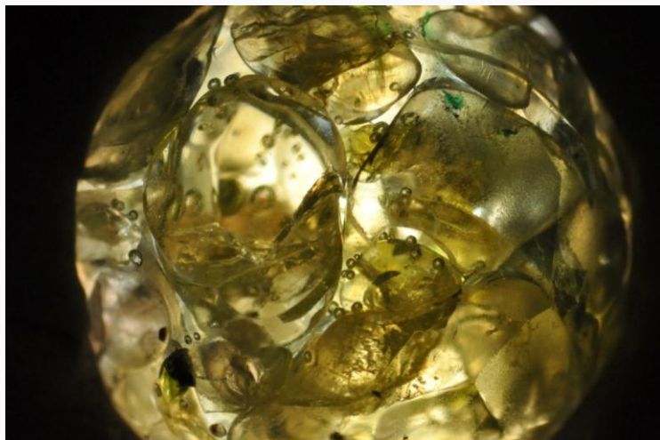
Figure 2: The bead in Figure 1 consisted of several pieces of yellowish green peridot embedded in a pale yellow polymer matrix. Note the presence of gas bubbles confined to the interstitial polymer areas. Magnified 24x.
