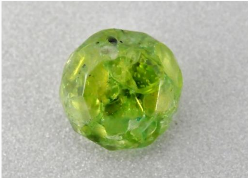
Figure 1: This 3.25 ct bead turned out to be a composite, made up of pieces of peridot embedded in a polymer matrix.
