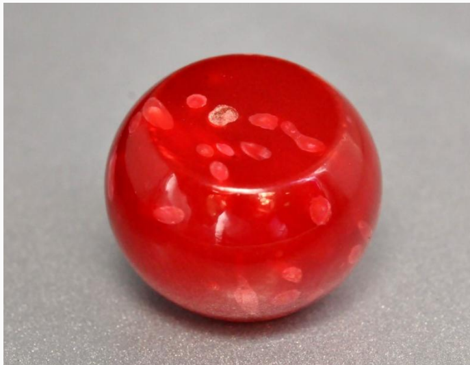
Figure 1: This 37.50 ct plastic bead contained visible fragments of carbonate-type coral (the lighter spots).
