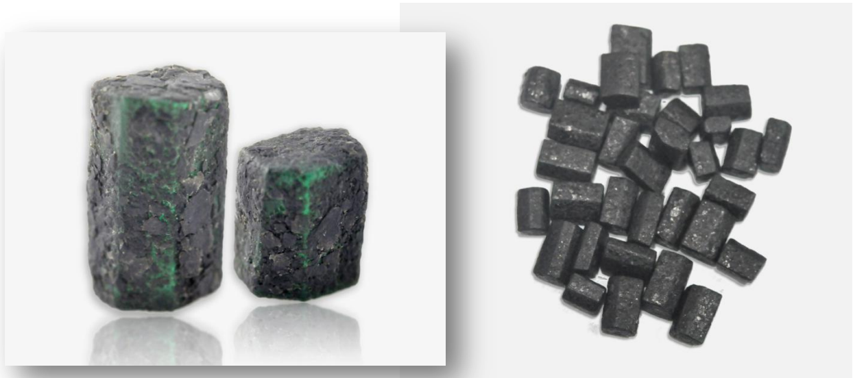
Figure 4: These glass samples worked-up to imitate emerald rough, are mixed in parcels of natural emerald
